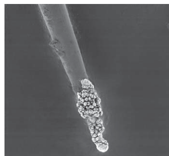
Figure 7. Low voltage image of an uncoated electrode with CNTs on tip. Imaged in SE mode. Magnification: 2,886x. Field Size: 140 \mu\text{m} . Courtesy of Plexon, Inc.
