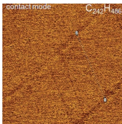
Figure 12. AFM images of C 242 H 486 lamellae on graphite obtained in the contact mode. Several slightly twisted lamellae were detected in the images of C 242 H 486 . A number of linear defects caused by the missing chains or their parts are also distinguished in the 100 nm image (left). The individual alkane chains, which are extended between the edges of the lamellae, are also noticed in the 55 nm image (right).
