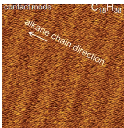
Figure 11. AFM images of C 18 H 38 and C 390 H 782 lamellae on graphite obtained in the contact mode. The spacings, which are related to the lamellae and individual chains, are distinguished in the image of C 18 H 38 lamellae (left). The zigzag pattern along the closely packed alkane chains is seen in the image of the ultra long alkane – C 390 H 782 (right).
