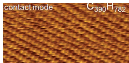
Figure 11. AFM images of C 18 H 38 and C 390 H 782 lamellae on graphite obtained in the contact mode. The spacings, which are related to the lamellae and individual chains, are distinguished in the image of C 18 H 38 lamellae (left). The zigzag pattern along the closely packed alkane chains is seen in the image of the ultra long alkane – C 390 H 782 (right).
