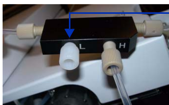
Figure 3 Dual AJS ESI source plumbed for high flow application
