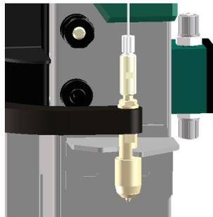
**2** Move the lift upward (arrow button **[Arrow up]**) until the needle or the filter is stripped off and falls into the collection container. Do not move the lift too far upward.
