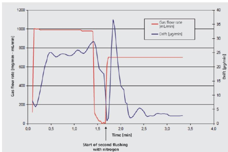
Typical gas flow rate and drift curves during water content determination in a liquid gas
