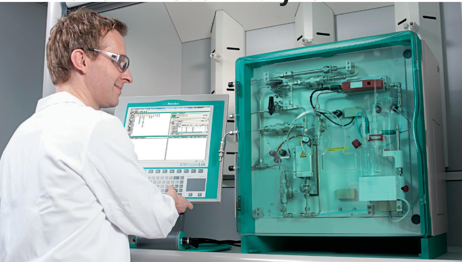
Coulometric water determination in liquid and permanent gases
