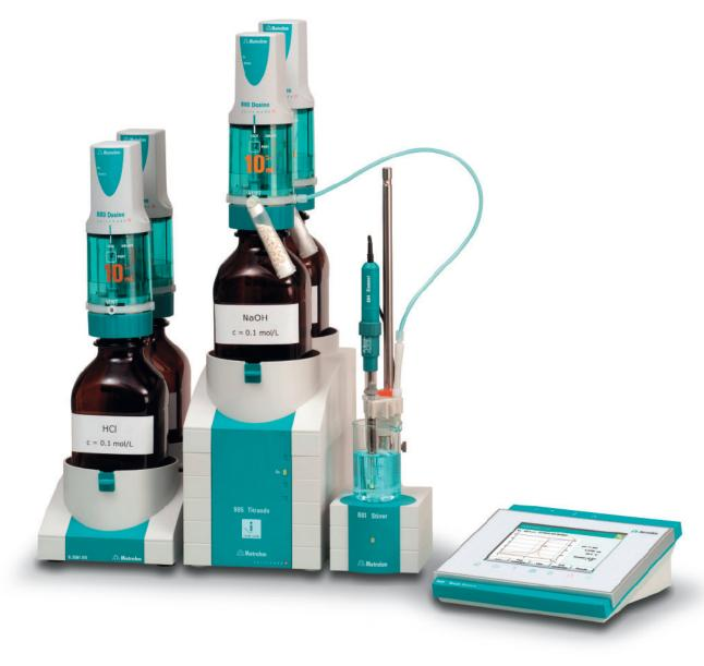
Increasing sample numbers, time-consuming sample preparation steps and unattended overnightoperation are good reasons for using sample changers. The 888 and 890 Titrandos have the necessary intelligence to control sample changers. Whether you require small or large sample capacity, one or two working stations, sample metering, sample preparation, liquid handling, rinsing
