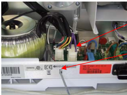
7890 - 3 Replace the transformer connectors and route the sensor cable through the rectangular hole.
