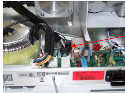
7890 - 2 Clip the oven sensor on one heater wire.
