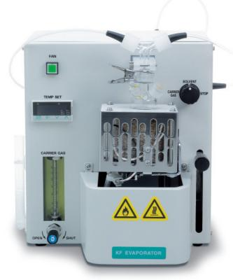
The oven is raised with a finger and the sample heated. Secondary reactions hardly occur, as the sample itself does not reach the titration cell.
