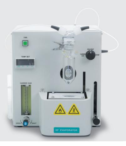
Sample preparation using azeotropic distillation in Karl-Fischer titration
