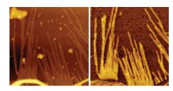
CdTe topography image (left) and (right) surface potential. Scan size  $1\mu m$ .
